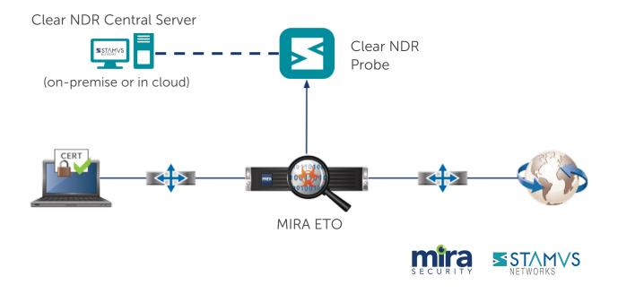
In a "network inline - appliance passive" configuration, the ETO sits in the middle of the traffic flow – between the client and the server. When the SSL/TLS handshake occurs, the ETO actively participates in the handshake to insert itself in the TLS flow, it then decrypts the flow and passes the plaintext data over to the Clear NDR Probe for analysis. Then it re-encrypts the data and sends it on to the destination, maintaining the end-to-end connection in an encrypted form.
